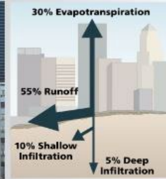
Figure 1. When roads, rooftops and parking lots cover much of the land, more than half of the rainfall runs off and flows directly into surface waters. In highly developed areas, such as in Seattle, Washington (above left), only 15 percent of rain water has the opportunity to soak into the ground.
